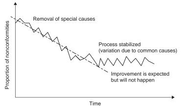
Figure 2.5 Stabilizing processes
