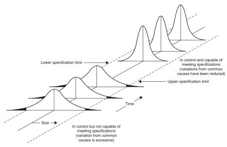
Figure 2.9 From process control to capable process
